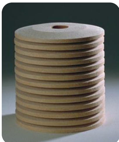
Micro-filter cartridge TFP 1000 heat-treated Dirt holding capacity: 2,000 g, filter fineness 3 \mu\text{m} absolute incl. set of seals
