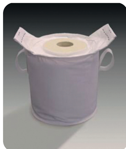
Combined micro-filter and drying cartridge CTFP 1000 heat-treated Dirt holding capacity: 1,100 g Moisture: 1,300 ml Filter fineness 3 \mu\text{m} absolute incl. set of seals
